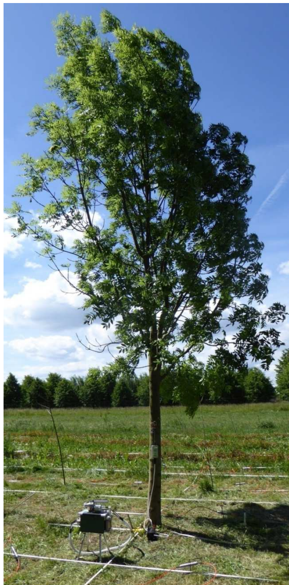
Figure 2. An investigation conducted by a complex of open field applicable methods on an Ash tree example. Visible: Sap flow meter (tree stem), portable photosynthesis system, electrical resistivity tomography electrodes (metal electrodes around the tree with orange wires) and soil moisture meter (in the tree shadow), during the site measurements.
