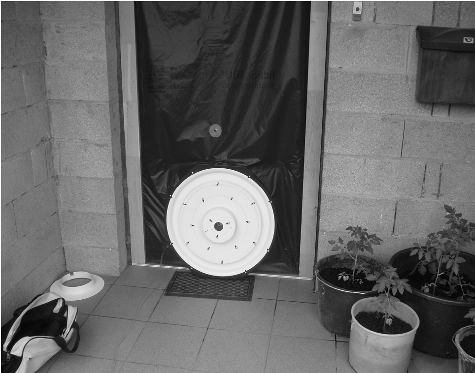
Fig. 1) Measurement of the building envelope air-tightness
