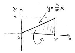
$$V = \pi \int_0^v \left(\frac{r}{v}x\right)^2 dx = \frac{\pi r^2}{v^2} \int_0^v x^2 dx = \frac{\pi r^2}{v^2} \left[\frac{x^3}{3}\right]_0^v = \frac{\pi r^2}{v^2} \frac{v^3}{3} = \frac{\pi r^2 v}{3}$$
